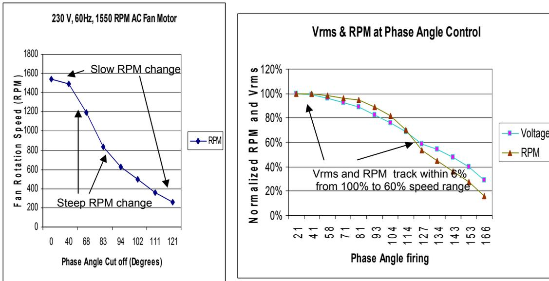
**Figure 2: Linear RPM Output Using Micro-control of TRIAC Phase Angle**
