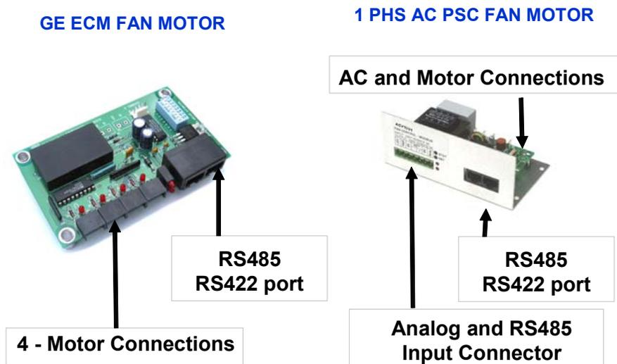
**Figure 5: Single-Phase PSC motor Controller and ECM 4-motor interface**
