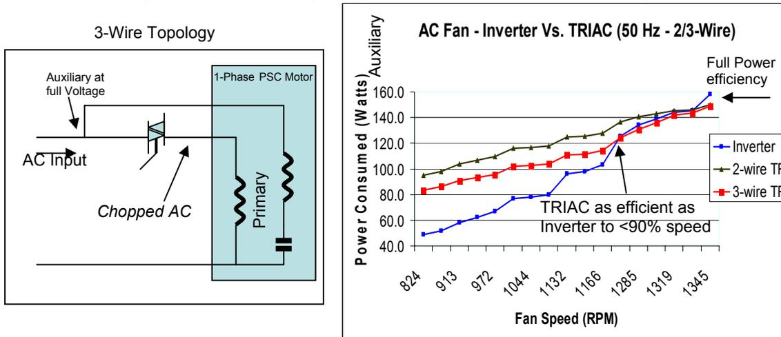
As can be seen by the above, the efficiency of the TRIAC control is improved and is competitive with Inverter solutions down to almost 90% of speed and continues to provide efficiency improvements through the normal operating range of fan control.
